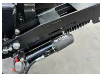
PLATFORM AUTOMATIC TILT TO THE GROUND WITH HYDRAULIC CYLINDER (NO ELECTRONICS AT ALL)
