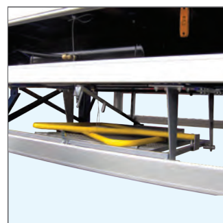
45 Structure to be fixed under the semi-trailer body to house 2 guards and the side ramp
