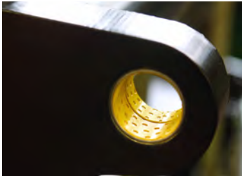
LOW MAINTENANCE BUSHES AND CHROMIUM PLATED PINS.
